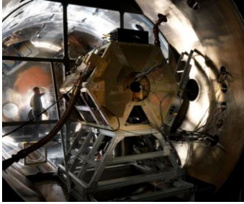
VX-200 engine (left), 200 kW argon plume (center) and measured and predicted performance data for Argon and Krypton
