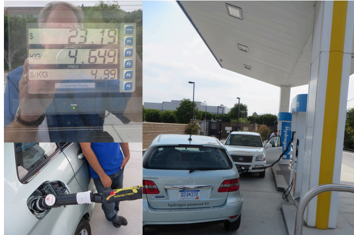
Hydrogen filling station, Torrance, California, two vehicles fill up with hydrogen in 5 to 10 minutes. Dispenser screen (top, left) shows full service cost (source: Ad Astra Rocket Company)
