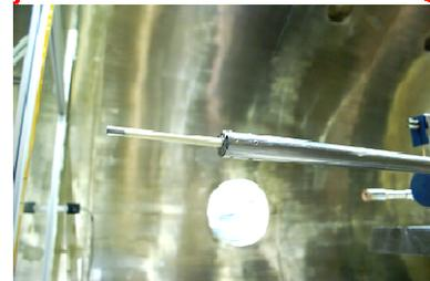
**Fig. 6. Photograph of the Langmuir probe with guard ring on a 70 cm extension shaft.**
