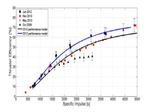
Fig-1: VX-200 engine performance over several experimental campaigns (2009 – 2012). Blue trace shows the new performance model based on the most recent data.
