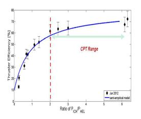
Fig-2: VX-200 engine efficiency vs second to first stage power ratio. Above a ratio of  $\ge$  2,throttling can be done without significant loss in efficiency.
