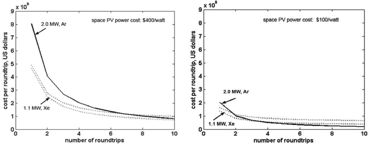
**Figure 5: Cost dependence of lunar cargo technologies on propellant cost, power cost and system lifetime.**
