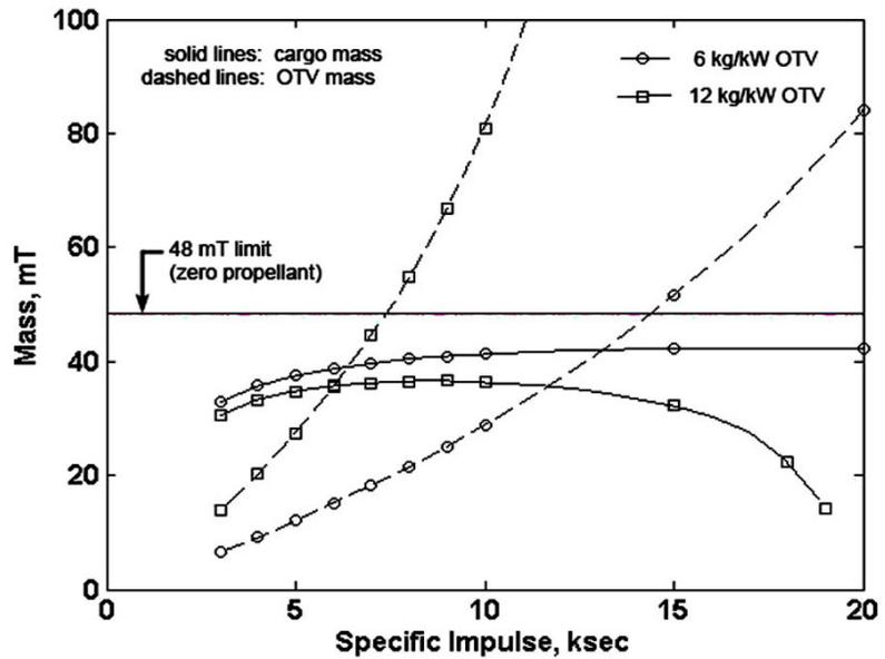
**Figure 4: Effect of specific mass ( $\alpha$ ) on cargo system performance. Transit time is 180 days.**
