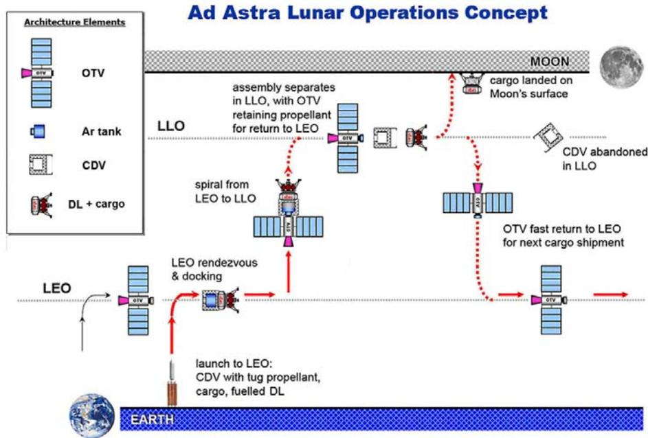
**Figure 1. Architecture of Lunar Cargo System.** The solar-powered VASIMR™ OTV (orbital transfer vehicle) is launched to low Earth orbit, followed by launch of a CDV (cargo delivery vehicle) for each round trip to low lunar orbit and back.
