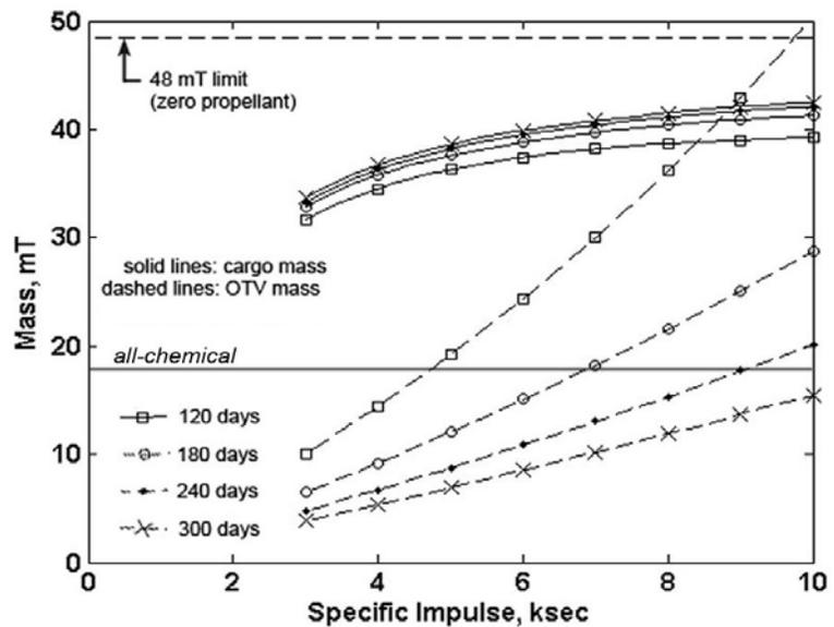
Figure 3: Effect of transit time on cargo mass and mass of the OTV (for  $\alpha = 6$  kg/kW).
