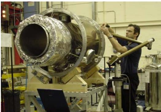
VX-200 superconducting magnet testing at Scientific Magnetics Ltd.
