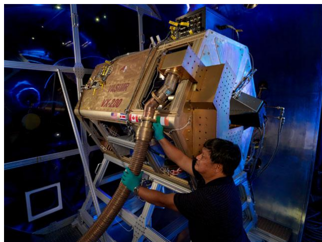
Figure 7. VX-200 ™ installed in Ad Astra's vacuum chamber.
