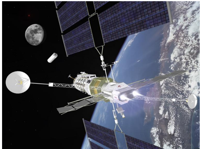
Figure 8. Artistic diagram of a 200 kW VASIMR ® -SEP spacecraft performing debris rendezvous.
