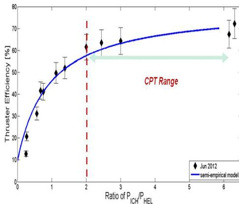
**Fig-2: VX-200 engine efficiency vs second to first stage power ratio. Above a ratio of  $\geq 2$ , throttling can be done without significant loss in efficiency.**
