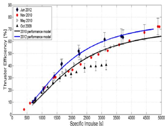
**Fig-1: VX-200 engine performance over several experimental campaigns (2009 – 2012). Blue trace shows the new performance model based on the most recent data.**
