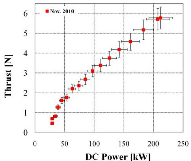
Thruster efficiency vs exhaust velocity (specific impulse x 10) and thrust vs input DC power. Results are shown for three separate experimental campaigns in October 2009, May of 2010 and November of 2010. Hardware refinements to the second stage have led to significant performance improvement.
