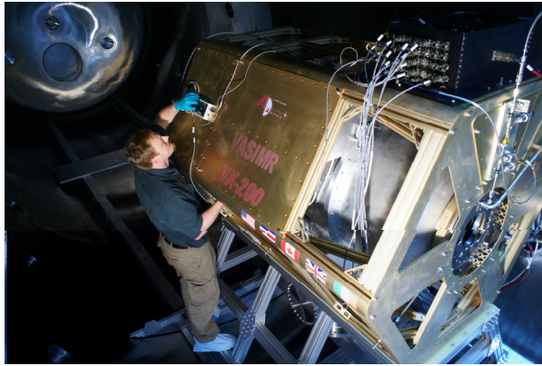
VX-200i undergoing vacuum chamber tests, Houston Facility.
