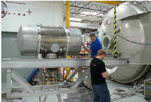
VX-200 Superconducting magnet is installed in test frame and undergoes magnetic field measurements.
