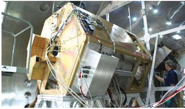
Figure 1. VASIMR® VX-200i prototype.
