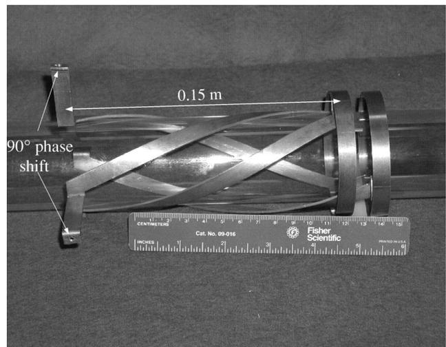
FIG. 2. A quad-phased antenna with  $90^\circ$  phasing between helical segments was used for most of the experiments and the modeling described in this paper.
